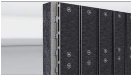
Fasten edge-clamps with stainless steel blind rivet (Art. no. 675)
