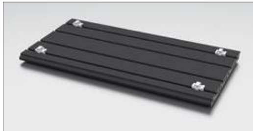
Push the adapters (Art. no. 596) in the grooves on the back – at least 4 adapters per panel
