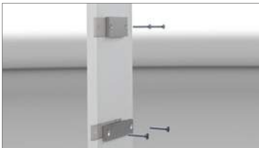
Fix base plate at the basic substructure
