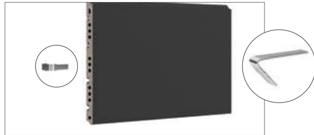
Hang the KeraTwin® panels with the adapters in the horizontal rails – for securing the position of the panels, use joint spacers (Art. no. 645)
