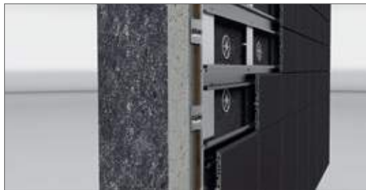
Hang the KeraTwin® panels with the adapters in the horizontal rails – for securing the position of the panels, use joint spacers (Art. no. 645)
